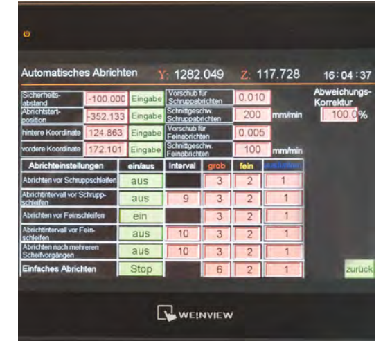
Dressing mode for grinding wheels with automatic dimension and speed (rpm) compensation ensures constant grinding rate and can be entered while in auto mode
