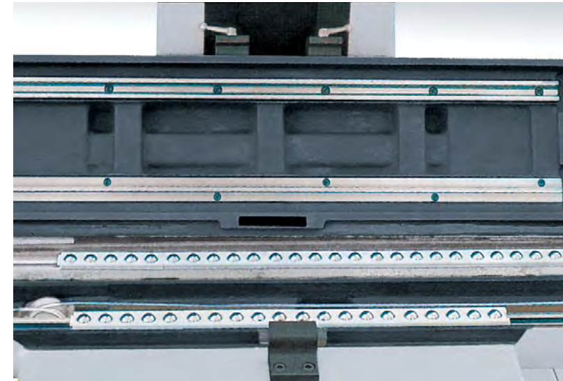
Linear ball guide for guide for smooth table travel
