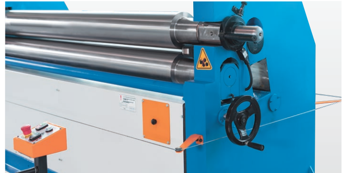
Upper roller can be swiveled out
