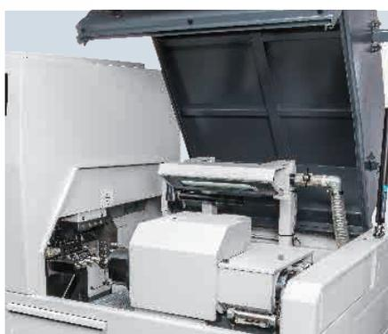
Elevating roof type protection door
