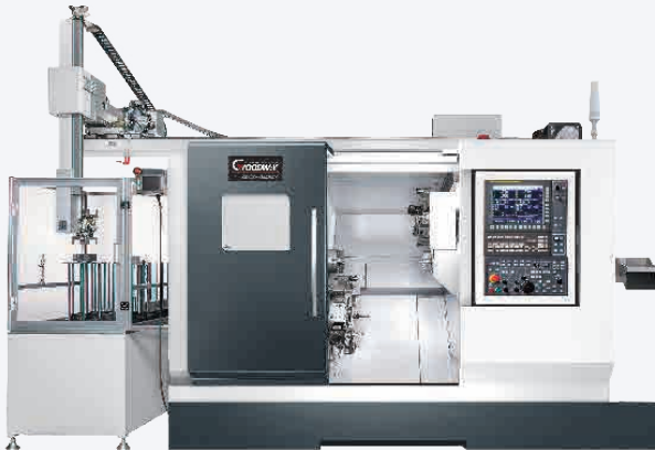
Twin Jaws Robot Arm
