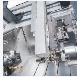
Twin Jaws Robot Arm
