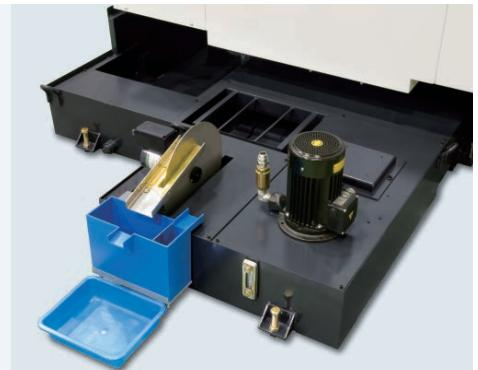
Separate coolant tank & Oil skimmer shown
