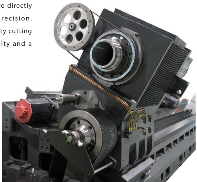
► The 2-speed, super heavy-duty gear head incorporates advanced mechanical designs. Mated with a 37 kW ( 30 min. ), a tremendous amount of low-end torque is provided to handle heavy material removal on large diameter parts.
