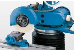
Surface grinder with angular adjustable vise
