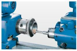
High-speed inside cylindrical grinding
