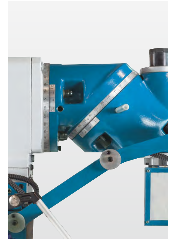
Cutter head swivels on 2 levels
