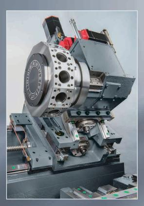
■ 30° slant bed design provides extremely stable base and saddle.
