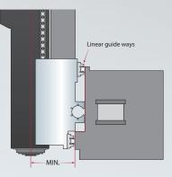
Y-axis sectional roller type guide ways design
